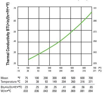
Thermal conductivity and physical properties based on unfaced mineral wool fittings. Technical data as supplied by Eagle-Pitcher.
